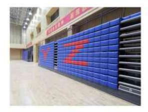
The stands are fixed against the wall. After these stands are completely folded, the whole group of stands is placed on the wall to free up space.
